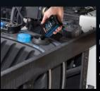
ONLY ADD TO ADBLUE® TANK Use at every refill of AdBlue® 500 ml treats 1 AdBlue® tank (45 to 75L) 125 ml treats 1 AdBlue® tank (10 to 20L)
